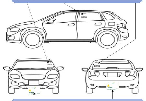
Licence plates to be displayed in a vertical position and firmly fixed to the outside of the vehicle at the front and rear, using the fixing bracket provided for the purpose. Velcro or cable ties are not permitted to be used
